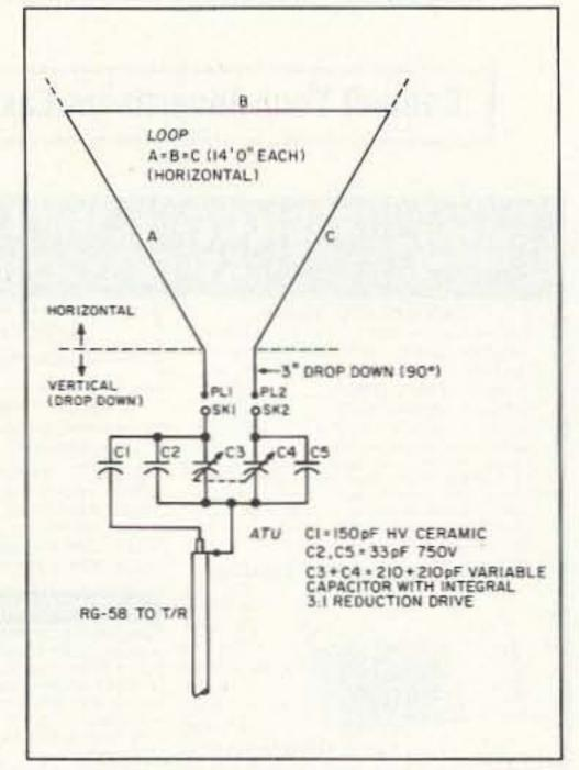
Figure 1. Diagram of the Compact-A-Loop.
